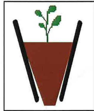
Incorrect - Narrow the shoe with adjustment bolt.
