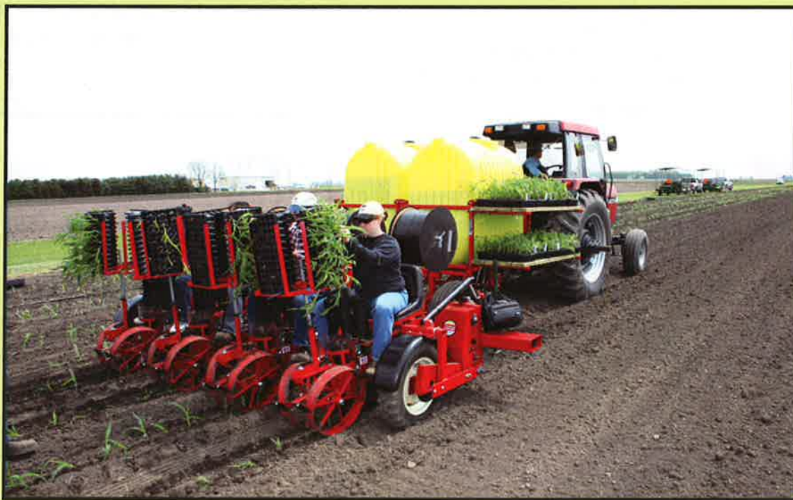
Model 803 4HF 5000W planting corn trials in Indiana. This pull-type 4-row is shown with two 300 gallon tanks and plastic tray carrouseles. Options shown: shelves on trailer saddle sides, four drip irrigation attachments and cushion seats.
