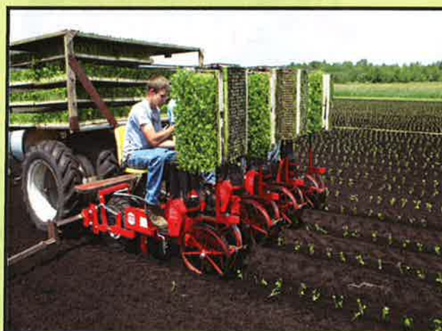
Model 5000WD 4 row planting celery with styrofoam trays behind self-propelled power unit
