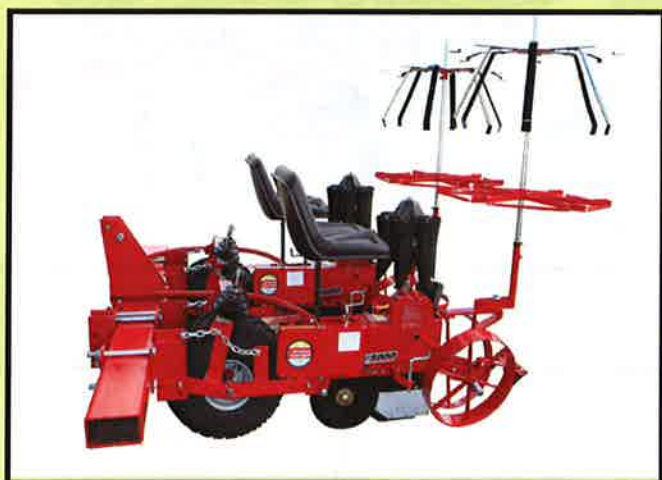
Model 5000WD 2 Row with optional cushion seats, 6 tray carrouseles and poly double disc shoes
