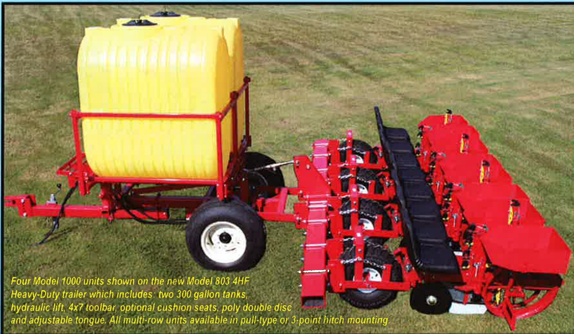
Model 803 2 1000 - Two row with NEW 803 heavy duty trailer. Shown with upright 300 Ga. tank, telescoping tongue, 4x7 toolbar and two Model 1000 units. Options: cushion seats, double disc poly shoes, rubber packing wheels and 7:60 x 15 tires.
